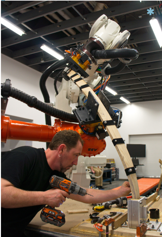
Multi-robot steam bending of timber elements with 6-IR camera-based real-time trajectory compensation
